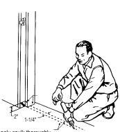
Apply caulk thoroughly to prevent water leakage
