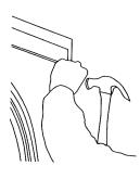
After the door is centered, anchor the door in place. First, nail through the metal door frame on the hinge side in the holes provided. Place a nail in the top hole of the lock side. Then close the door and eye the margin down the side, you may need to tap the frame a little to adjust it.
