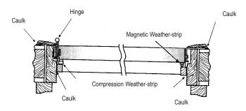
Install the hinge side compression type weather-strip in the same way you installed the lock side. Remember to first tack, make adjustments, and finish nailing.
