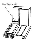
Peel the paper backing off and place these on the bottom of the jamb against the threshold as shown.
